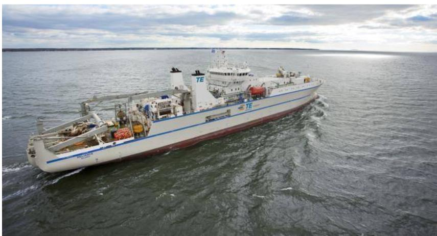
**Figure 5. TE SubCom's Reliance Class Cable Installation Ship**
