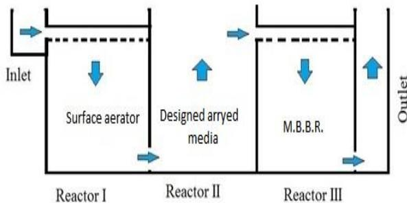
Figure 1 - Schematic Representation of Longitudinal Section of Model
