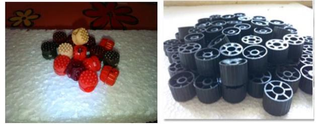
Figure 2: Photographic Representation of Anox Kaldnes biofilm carriers and MEDIA I.
