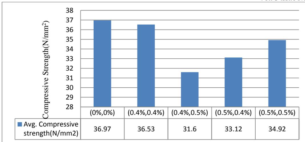
*Figure 3: compressive strength (28 days)*
