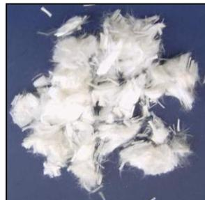
*Figure 2 Polypropylene Fiber*
