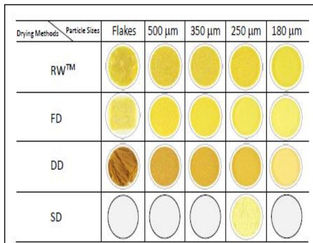
**Fig.9. photographs of mango flakes or powder at different particle slices obtained from different drying methods. - Adapted from O.A. Caparino *et al.* (2012)**
