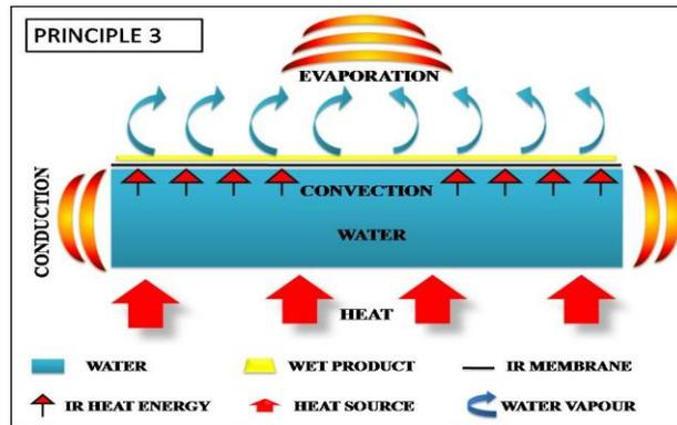
*Fig.4. Principle 3 – When wet product is applied uniformly on IR membrane*
