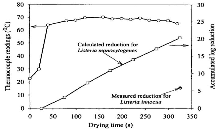
**Fig.8. Puree temperature and accumulated log reduction in population of *Listeria Monocytogenes* as a function of drying time**
