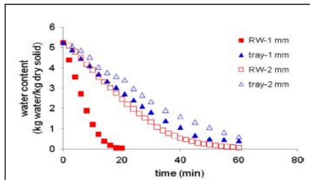
**Fig.7. Kinetics of moisture content for RW and tray drying at 90 °C for 1mm and 2 mm samples (C.I. Ochoa-Martínez et al. 2011)**
