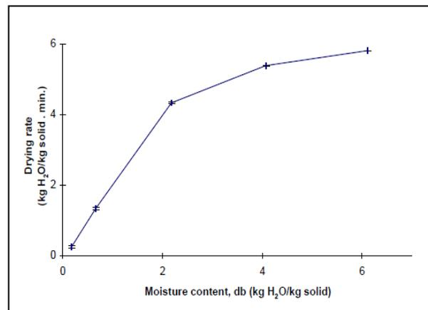
**Fig.6. Refractance window drying curve for carrot puree-drying rate v/s moisture content (Abonyi *et al.* 1991)**
