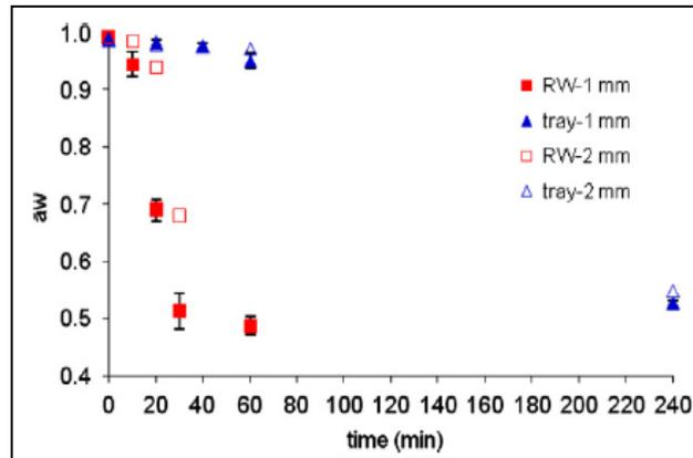
*Fig.10. Water activity behavior for RW and tray drying for 1 mm and 2 mm of mango slices (C.I.Ochoa-Martinez,2012)*
