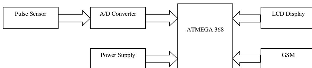
**Figure 1. Block diagram of Cuffless Blood Pressure Monitoring System**
