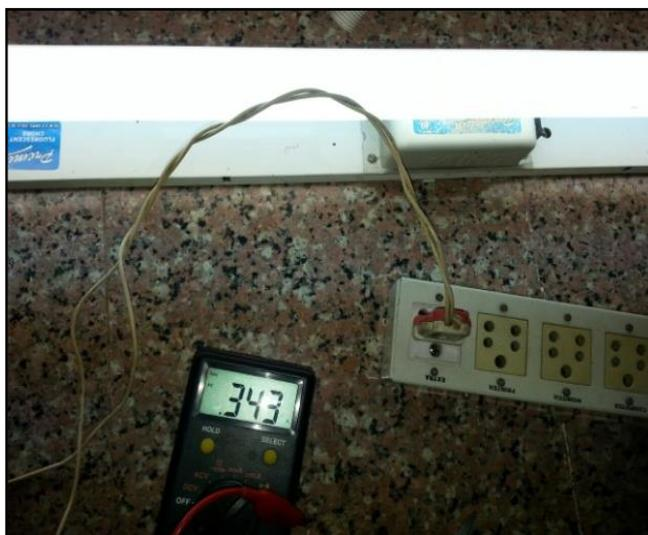
**Figure 4. Magnetic ballast current reading**
