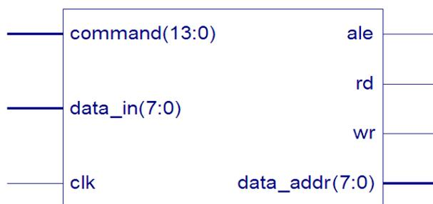
**Figure 12: RTL schematic for External memory interface module**
