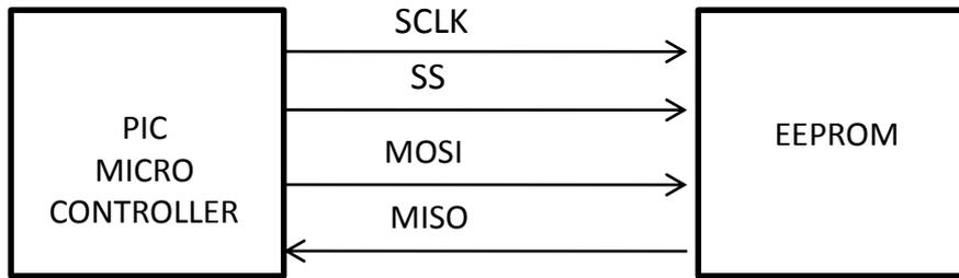
**Figure 2: Interfacing using SPI communication [3]**
