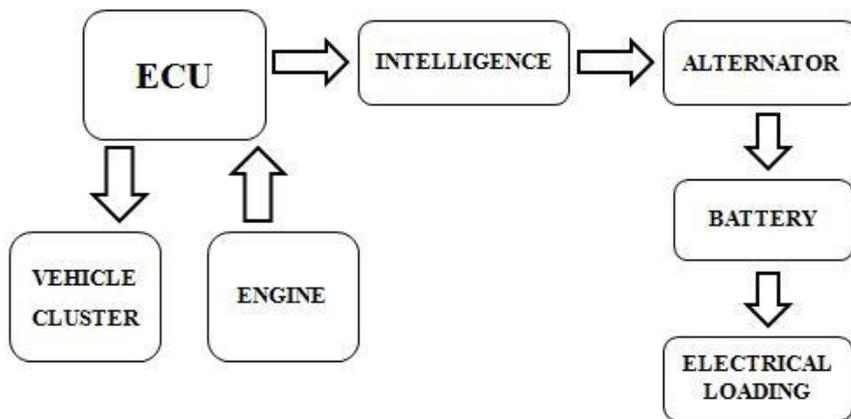
**Fig. 5 (a) Block diagram of intelligent alternator system**
