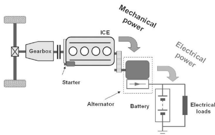
**Fig. 1 Alternator working scheme**
