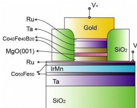
**Figure 6. Layer structure of MTJ sensor using MgO [17]**
