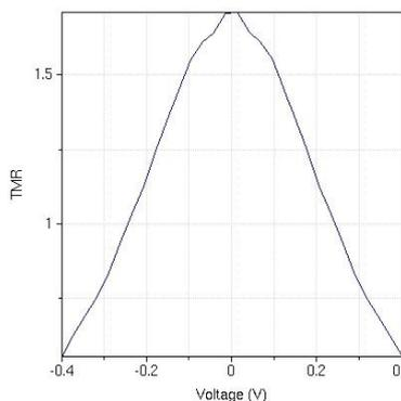
**Figure 9. Tunnel magnetoresistance (TMR) variation with applied voltage**
