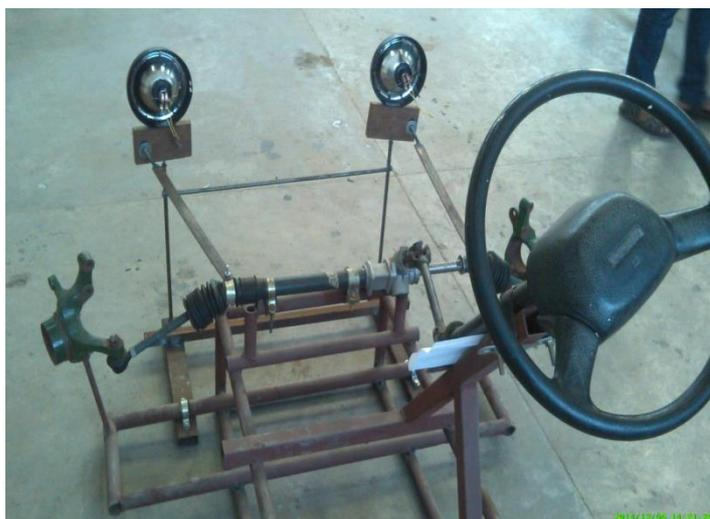
Figure 4. Movable headlights with Steering System
