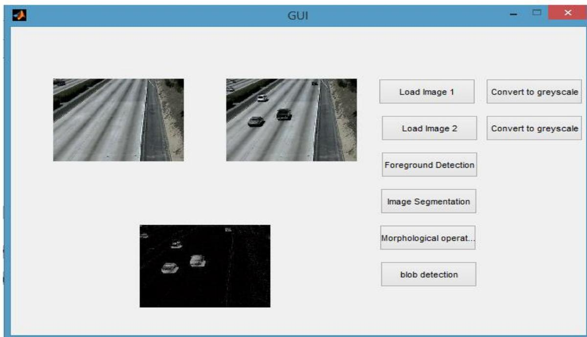
**Figure 3. GUI performing Image subtraction**
