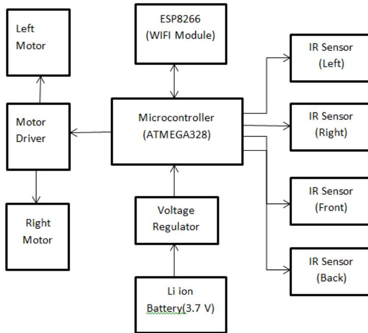
Fig 1. Block Diagram Of Micro Robot
