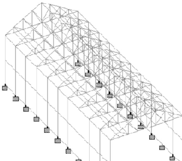
Fig: 3 Structure of roof truss from STTAD Pro [ Refer from STAAD Pro]
