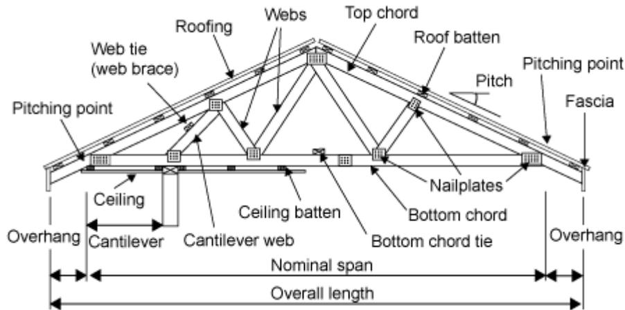
Fig: 2 Components OF ROOF TRUSS [Ref no. 9]
